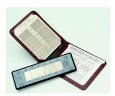
Comparators allow the estimation of surface roughness, by both touch and sight.
