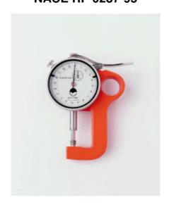
The Elcometer 124 Thickness Gauge issued to measure the peak-to-valley height of a surface profile formed in the Elcometer 122 Testex Tape.
