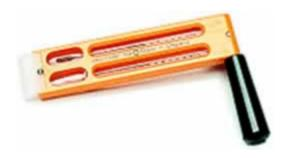
The Whirling Hygrometer employs the wet and dry bulb principle to determine the relative humidity of the atmosphere. The instrument consists of wet and dry bulb thermometers mounted side by side in a frame with spindle and handle attached.
