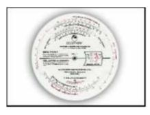
This provides accurate values of Relative Humidity (RH) and dewpoint from the wet and dry bulb temperatures of a Whirling or Sling Hygrometer - such as the Elcometer 116 range.
