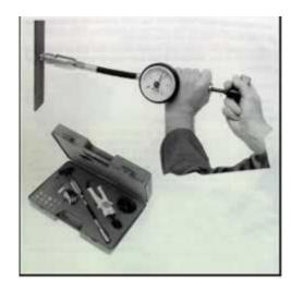
The Elcometer 108 is an extremely versatile hydraulic adhesion tester which will cope with virtually any adhesion test requirement. Tests can be made on flat, concave and convex surfaces and the instrument can be operated at any angle.
