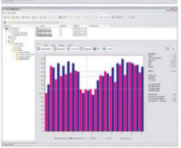
The software has been designed to be familiar and intuitive to any PC user. When the gauge is connected to the PC, individual readings can be sent directly into the software for real time analysis or simply 'drag and drop' a batch from the gauge to the software.
