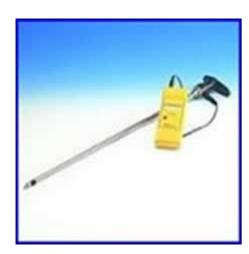
The Digital balemaster is a hand held instrument which displays the results on a large LCD Digital Display. The probe is made from strong durable stainless steel and is 600 mm long to reach the centre of big bales
