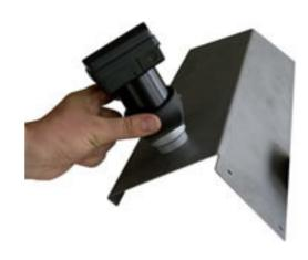
The **Affri Metaltest** is a portable Rockwell Hardness tester with direct digital read-out. It is designed for hardness tests on particularly cumbersome items, materials in the warehouse, and pieces which cannot be tested on a bench Hardness Tester.
