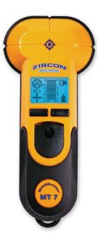
MetalliScanner MT 7 metal detector quickly and easily locates rebar, pipes, and other metal before you saw or drill. The bright, backlit display indicates metal target depth up to 152mm deep, type of metal located (ferrous or non-ferrous) and whether you are moving towards or away from a target. Use to find and avoid rebar in concrete before drilling, to find pipes and junction boxes behind tile, and even detect the nails/tacks in studs behind lath and plaster walls.
