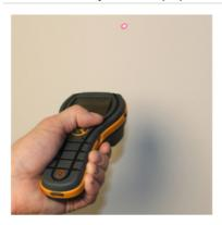
Checks surface temperature, utilizing laser pointer, calculates proximity to dewpoint
