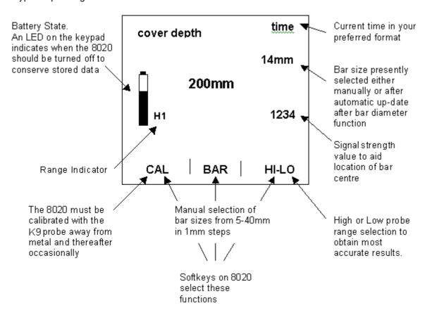
On/Off-Function switch on keypad selects Menus as required. The screen appearing immediately after the Cover depth screen shown above is for Bar Sizing. A further screen is available for examining data that has been logged from the K9 probe. This probe also has an LED for assisting in finding the top dead centre position of bars as the probe is swept across the surface.
