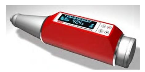
HT-225D is an integrated digital concrete test hammer which combines a data processor and a test hammer into one unit. It is widely used for non-destructive testing the quality of concrete and building materials in a finished structure or in prefabricated blocks. From its rebound value, the compressive strength of concrete can be calculated automatically. All testing data can be stored in the memory and transferred to a PC using a USB cable or wireless via Bluetooth.
