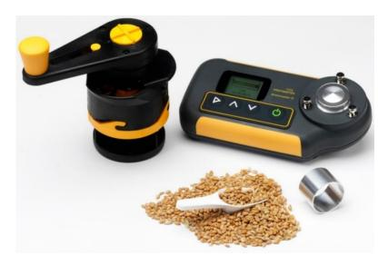
Protimeter Grainmaster i2 ® uses the ground grain moisture testing method for unrivaled repeatability and accuracy. It can also be used with optional probes to measure temperature in grain, as well as moisture in hay and straw.
