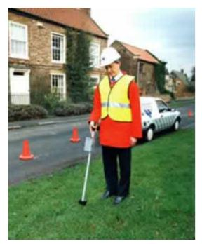
Live cable locators can only find electrical cables that have a current flowing through them to a depth & radius of 5 metres. They will not locate cable through which no power is being drawn.
