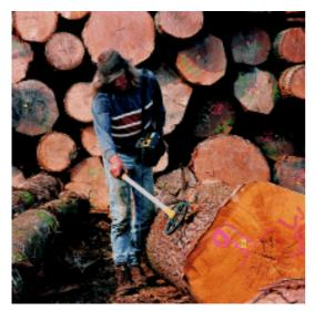
The Elcometer P610 has been designed specifically to accurately locate ferrous metal objects - such as gate hooks, nails, staples and even shrapnel - in timber, logs and wood of all types.
