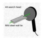
Approximate detection ranges: Mild steel / galvanised fishtail: 130mm Also used in the Timber Industry
