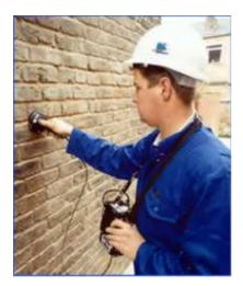
The Elcometer P130 will rapidly and precisely locate mild steel or stainless steel wall-ties and also makes an excellent stud locator / stud detector, it is therefore an extremely versatile instrument.
