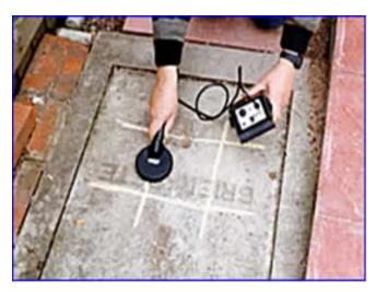
The **Elcometer P100** is a robust and economical gauge designed to identify the location and orientation of reinforcement bars, metal gas and metal water pipes.
