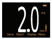
All gauges have a fully customisable, scratch and solvent resistant colour LCD display. Measurement modes available include Pulsed-Echo (P-E), Echo-Echo ThruPaint™ (E-E) and Velocity mode (for more information on measurement modes, see page 19). A choice of measurement units is available, depending on the measurement mode selected. A stability indicator shows clearly both the strength and reliability of the ultrasonic signal.
