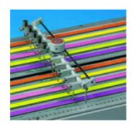
Designed to determine paint drying time by linear recording, with up to 10 test positions. Ten rods with hemispherical tips, fitted to a carriage, are brought into contact with the fresh film from one end of the test piece and moved lengthwise on the samples. The drying time is calculated from the distance travelled, measured using a graduated rule along the edge, corresponding to the various stages observed on the trace.
