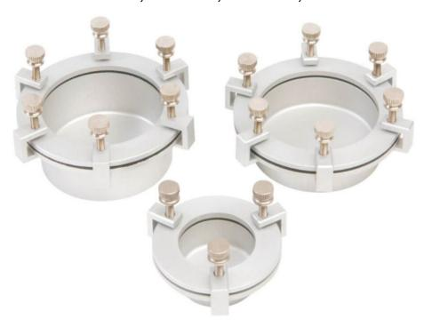
The Elcometer 5100 Payne Permeability Cups are made entirely from anodised aluminium and are used to determine the permeability of films of paints, varnish, plastic, cellophane, etc.
