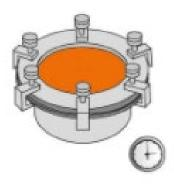
Leave for appropriate time, reweigh, calculate the change in mass  $(\Delta m)$  & water vapour transmission rate.
