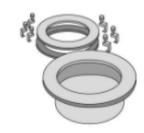
Disassemble the permeability cup
