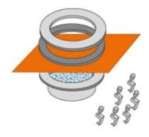
Place the film on to the cup and reassemble making sure the gasket is fitted.
