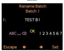
Stores individual adhesion strength readings and pull rate graphs in up to 2,500 alpha numeric batches, together with date, time and attribute information.
