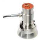
When testing coatings on low bond strength substrates such as concrete, wood or other fibrous materials, a larger surface area of dolly (50mm) is required to provide accurate, repeatable and reproducible results. The Elcometer 510 is available as a Concrete Adhesion Tester Kit, or 50mm accessory items (skirt, dolly, cutter) can be added to existing Elcometer 510 adhesion kits
