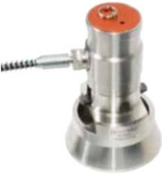
When testing coatings on low bond strength substrates such as concrete, wood or other fibrous materials, a larger surface area of dolly (50mm) is required to provide accurate, repeatable and reproducible results. The Elcometer 510 is available as a Concrete Adhesion Tester Kit, or 50mm accessory items (skirt, dolly, cutter) can be added to existing Elcometer 510 adhesion kits
