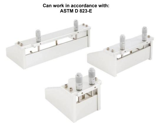
The Elcometer 3580 Casting Knife Film Applicator is available in a wide range of film widths and has extended sides to confine the coating during the application and is an ideal gauge for the laboratory.
