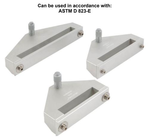
The Elcometer 3570 Micrometric Film Applicator is made of anodised aluminium with a reservoir and a bevelled blade applicator body and is suitable for high-precision manual application of high viscosity fluids onto relatively firm substrates.
