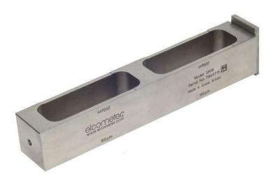
The Elcometer 4 Gap Film Applicators are precision engineered from hardened stainless steel to provide four film thicknesses in one gauge.
