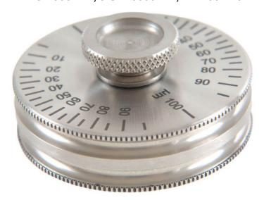
This instrument is similar to the Elcometer 3230 Wet Film Wheel, but is designed for use in the coil coating process.
