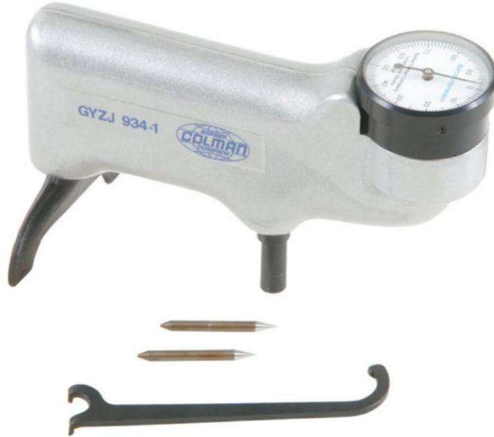
The Elcometer 3101 Barcol Impressor Hardness Tester is an easy to use hardness tester, ideal for measuring hardness of soft metals, plastics, glass fibre and leather.
