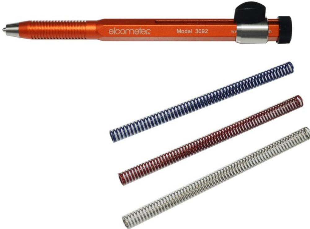
The Elcometer 3092 Sclerometer Hardness Tester measures the hardness of a coating by moving a Tungsten Carbide Tip over the coating with predetermined force.
