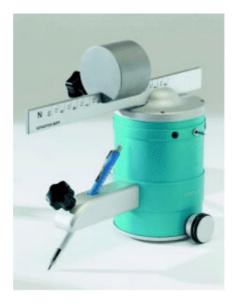
Similar to the **Elcometer 501** and using the same pencil technique, this motorised device in anodised aluminium can travel forwards (chip method) or backwards (indentation method) at a uniform speed further increasing the reproducibility of the test.
