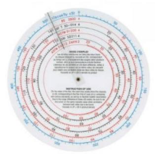
A conversion table that allows the viscosity (in cSt) and flow times of different cups to be compared.
