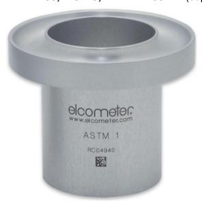
Viscosity Flow Cups are very easy to use instruments made of anodized aluminium with a stainless steel orifice, for measuring the consistency of paints, varnishes and similar products. The measured kinematic viscosity is generally expressed in seconds(s) flow time. If the Standards stipulate conversion methods the flow time can be converted into Centistokes (cSt) using the Elcometer ElcoCalc™ Mobile App.
