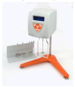
The Elcometer 2300 Rotational Viscometer range measures the viscosity of liquids in accordance with several standards. Using a rotational viscometer, the properties of liquids and their resistance to shear or flow can be accurately measured.
