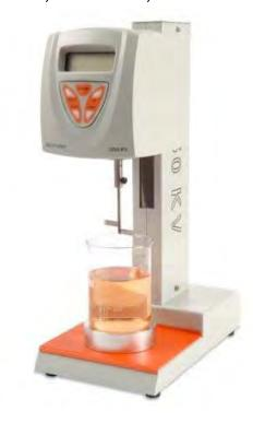
Featuring a unique automatic test mode, the Elcometer 2250 Krebs Viscometer measures the viscosity of paints, varnishes, adhesives, pastes and liquid inks at the touch of a button.
