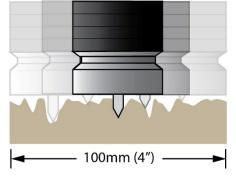
1. Ensure probe is 90° to substrate to ensure accurate readings and calibrate the gauge on a glass zero tile.
