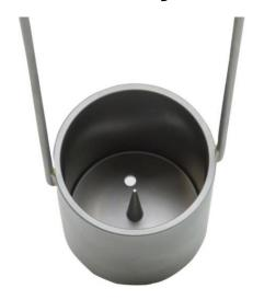
The Elcometer 2215 Lory Viscosity Cup is a conventional cylindrical cup with a needle fixed into the bottom for quick measurements on-site or during production.
