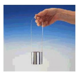
Conventional cylindrical cup with a needle fixed into the bottom for quick measurements on-site or during production.
