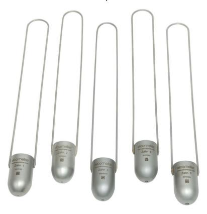
The Elcometer 2210 Zahn Dip Cup is a small U-shaped cup suspended from a looped wire. This method is ideal for measuring the consistency of paints, varnishes and similar products.
