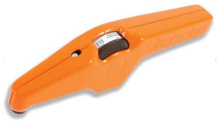
The Elcometer 211 Coating Thickness Gauge, commonly referred to as the "Banana Gauge", is a Type I instrument designed to measure dry film thickness.
