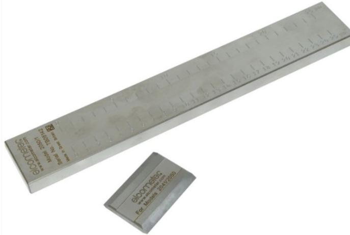
This single channel precision grind gauge is used to determine particle size and fineness of grind for many materials including paints, pigments, inks, coatings, chocolates, and other similar products.
