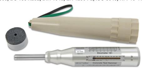
The concrete test hammer provides a quick, simple and inexpensive method for non-destructive evaluation of concrete compression strength and other masonry materials.
