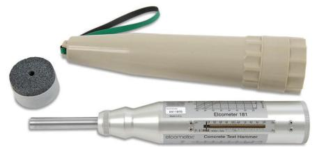
The concrete test hammer provides a quick, simple and inexpensive method for non-destructive evaluation of concrete compression strength and other masonry materials.
