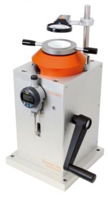
This robust and user-friendly tester is used for assessing the cupping ability of coatings applied to metal sheets up to 1.2mm thick.
