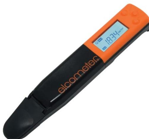
Incorporating a flat sensor, the Elcometer 138 Bresle Salt Meter measures the conductivity of a sample, then automatically converts this to show the density of salts, negating the need for the user to do a manual calculation when working in accordance with ISO 8502-6 or ISO 8502-9.
