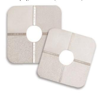
These extremely durable surface comparators allow the estimation of surface profile of either grit or shot blasted surfaces. Using the Elcometer 125 surface comparators as a reference the blasted profile can be compared to the four reference profile grades in each comparator. Profiles are recorded in microns. 4 Profile Values per Comparator.
