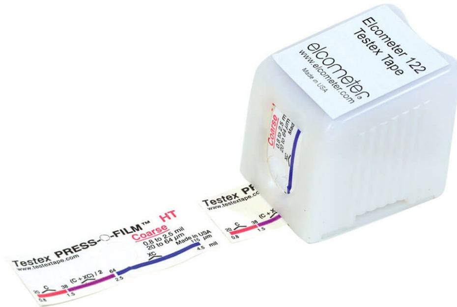
The proper and effective preparation of a surface prior to coating is essential. Making sure that the correct roughness – or profile – has been generated is essential. If the profile is too low, the adhesion of the coating to the surface will be reduced. Too high and there is the danger that the profile peaks will remain uncoated – allowing rust spots to occur.
