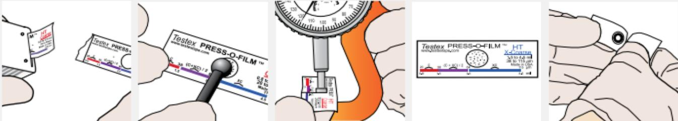
1. Tear off one section of the tape from the roll, peel off the backing tape and retain the back if required for future use.
