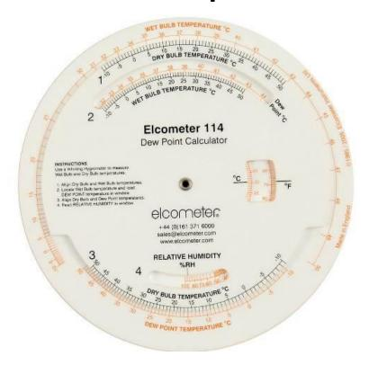
The Elcometer 114 Dewpoint Calculator provides accurate values of Dewpoint and Relative Humidity (RH) from the wet and dry bulb temperatures measured by a Whirling or Sling Hygrometer.
