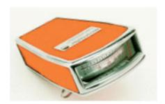
The Elcometer 101 was the world's first portable coating thickness gauge, first produced in 1947 and still has some advantages over other gauges
