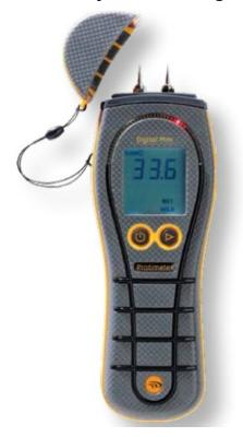
The Digital Mini allows building professionals—such as flood damage restoration contractors, surveyors, homebuilders and architects—to assess building moisture levels during new build and refurbishing activities. Excessive moisture in buildings can lead to decay and deterioration of components and decorative finishes. Professionals involved with the identification, management and remedy of moisture need tools that help them to:
