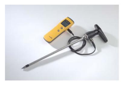
The Digital balemaster (GRN 6160) is a hand held instrument which displays the results on a large LCD Digital Display. The probe is made from strong durable stainless steel and is 600 mm long to reach the centre of big bales
