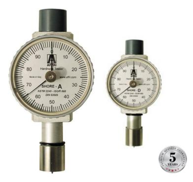
This portable hardness tester, tests by using a point which penetrates the material under spring pressure, with variable force depending on the model. A direct reading is displayed on the dial which is graduated from 0 to 100 Shore Hardness Units.
